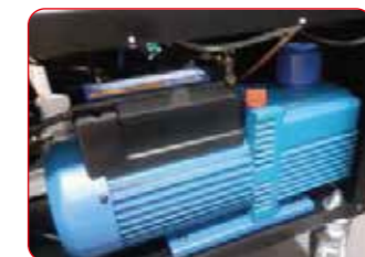
Strong Vacuum pump 142 l / min double stage
