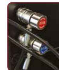
Quick couplers SAE J639 Hybrid function
